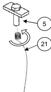
8.- In the larger hole also insert 3/8 x 1 1/2" bolt plate, but without using 3/8" bolt guide, Make sure they are as **PICTURE 6.**
