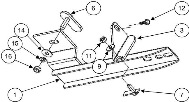
7.- Locate the holes in the rear of the chassis as shown in the **PICTURE 5**. Insert 3/8" bolt guide in 3/8 x 1 1/2" bolt plate, tuck the larger hole and pull the small hole. **SEE ILLUSTRATION 2, PICTURE 5.**
