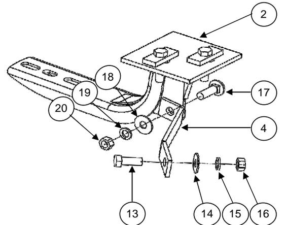
11.- Make any final adjustments to the alignment of the bracket and tighten all bolts.
