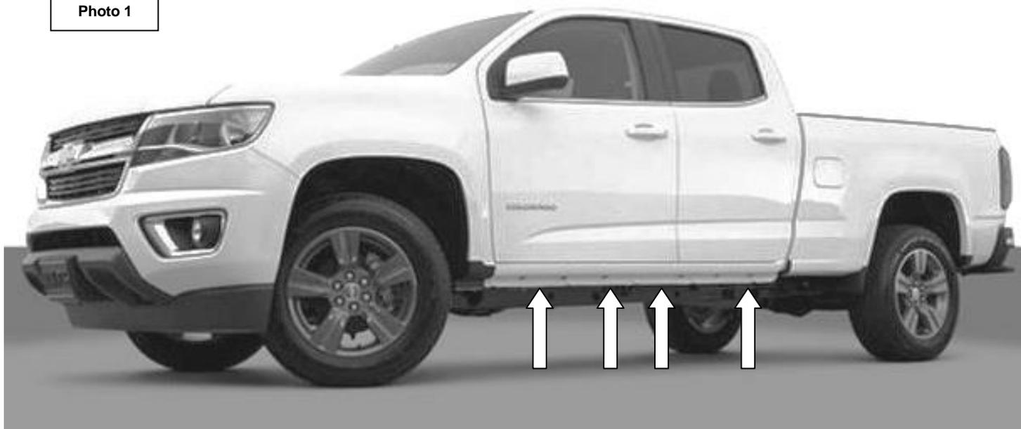
**Step-1** Begin the installation on the driver side. Starting at the front of the vehicle, locate and remove the plastic plugs in the back side and bottom of rocker panel to expose the holes used for placement of the M8 Clip- Nuts, (Photo 2).
