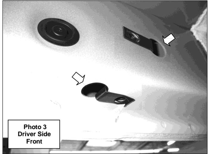
**Step-3** Attach one of the brackets to the rocker panel using (2) C/HEX SEMS M8X30MM P1.25 (Photo 4 & 5). Leave the bolts loose for final adjustment.
