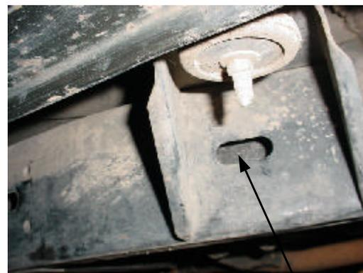
Introduce here a 1/2 x 1 1/2" cut carriage head bolt
