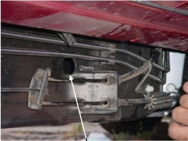
Insert in this hole the 1/2" bolt plate
