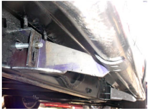
Rear bracket installed. (Passenger side).
