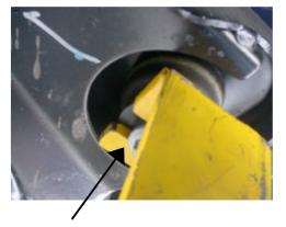
Existent bolt, untighten enough to locate the bracket.
