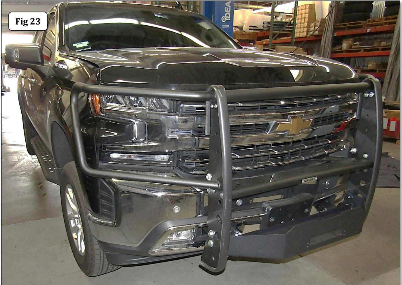
**Step-19** Attach the driver side headlight protector (not shown) to the brush guard using (1)  $\frac{1}{4}$ " x  $\frac{3}{4}$ " button head bolt, and the opposite end to the side plate using (2)  $\frac{5}{16}$ " x 1" button head bolts, (2)  $\frac{5}{16}$ " flat washers and (2)  $\frac{5}{16}$ " lock nuts. Repeat for the passenger side headlight protector. Align the grille and brush guard assembly, and tighten all nuts and bolts.
