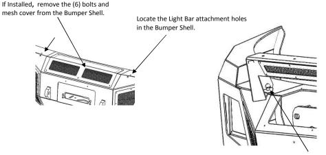
Secure the Light Bar to the Bumper Shell using (4) 3/8" x 1 1/4" hex bolts, (8) 3/8" flat washers, (4) 3/8" lock washers, and (4) 3/8" hex nuts.
