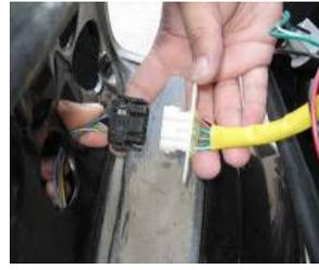
Step 7: Plug the wire harness into the new Anzo lights.
