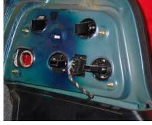
Step 3: Locate the four 8mm screws and remove them
