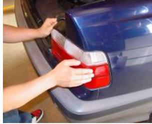
Step 6: Put the new Anzo light in and screw on the 8mm nuts to secure the tail
