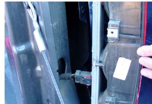
Remove the two torque screws that hold the taillights assembly to the truck.
