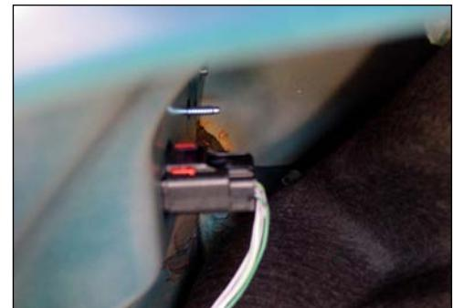
Insert the taillight onto the car and connect the stock plug in into the L.E.D. taillight. Make sure red clip is secure.
