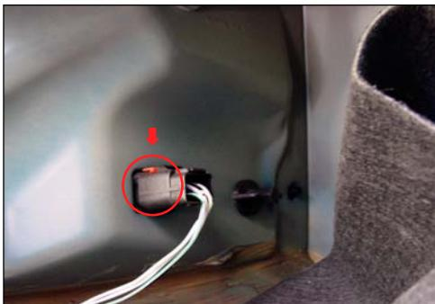
Pull the red clip out and disconnect the plug from the housing. Pull the taillight straight out.
