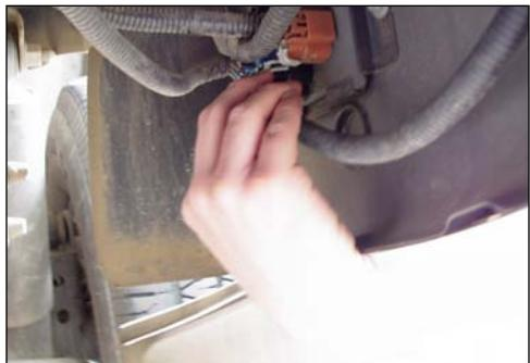
Disconnect the plug from the circuit board on the passenger side located above the tail pipe.
