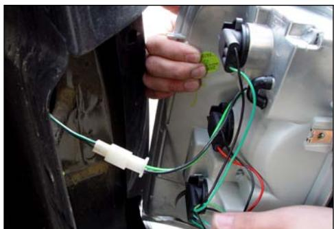
Connect the resistors to the wire harness. Make sure they are plugged in securely.
