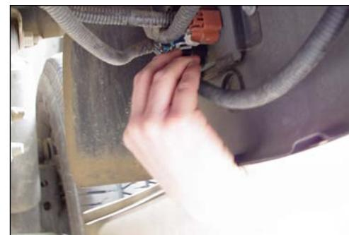
Connect the new wire harness to the circuit board underneath the vehicle. Make sure all functions are working properly before driving.
