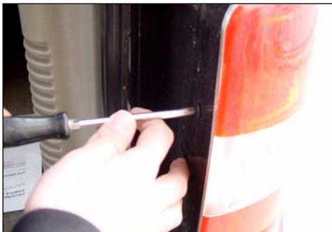
Remove the two phillip head screws that hold the taillight in place. Pull the taillights straight out.
