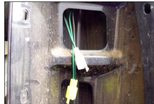
Install the resistor boxes in a location out of the way of the taillight housing.
