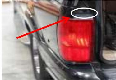
Remove 2 7mm torx wrench screws located on the top of the tail
