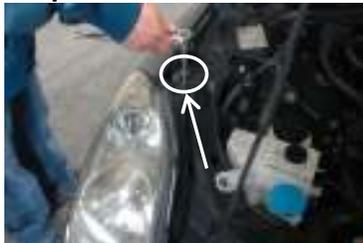
Remove (1) 10mm bolt located on top of the headlight.
