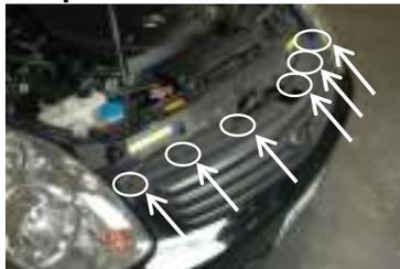
Remove (6) push pins located on top of the grill.
