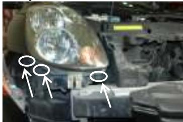
Remove(3) additional bolts from the headlight located on the bottom.
