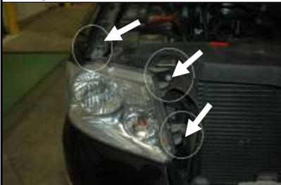
You'll need to remove the (3) 10mm bolts located on the top and side of each headlight.
