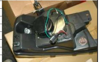
Splice the black (ground) and green (power) wires into the parking light circuit to power the LEDs and U-Bar.
