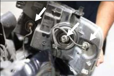
Gently pull the headlight toward you exposing the harness. Disconnect the each connector to remove the headlight from the vehicle.
