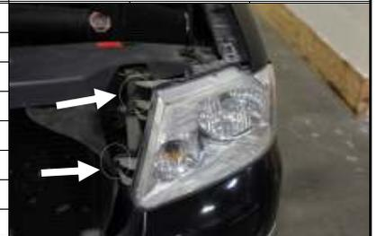
Remove the grille shroud to expose the (2) 10mm bolts on the side of the OEM headlight.
