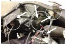
Remove the headlight by unplugging the power source and each of the three light bulb harnesses
