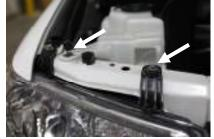
Remove the two 10mm screws located at the top of the headlight housing
