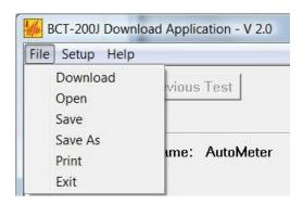
1. Download. This option will download the data from a BCT200J and save the data to a text file on the PC. Before choosing this option connect the round 6 pin plug of the AC-10 cable into the jack at the top of the BCT-200J. Connect the 9-pin DB connector of the AC-10 cable to a serial port on the computer.
