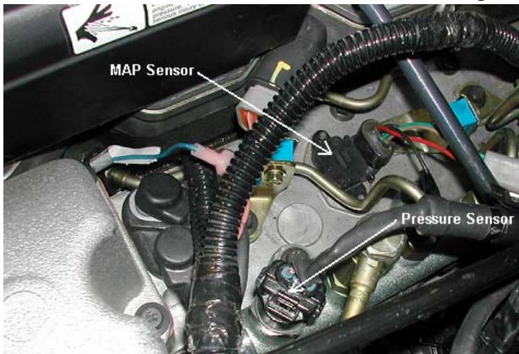
Disconnect the stock wiring harness at the sensor located on the main fuel rail on the driver's side towards the rear of the engine. Plug the supplied pressure sensor connector into the stock pressure sensor on the engine and the stock engine wiring harness connector into the supplied pressure sensor connector.
