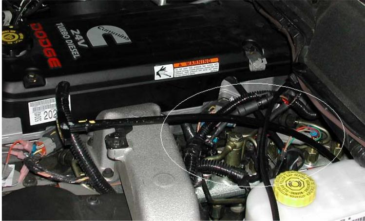
Disconnect the stock wiring harness at the MAP sensor located on top of the intake manifold. Plug the supplied MAP sensor connector into the stock engine MAP sensor and the stock engine wiring harness connector into the supplied MAP sensor connector.
