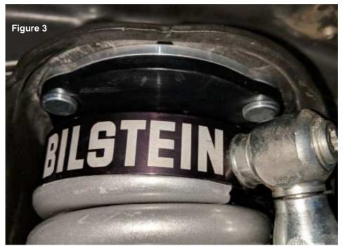
Note: The top mount spacer and spring depicted differ slightly in appearance from the supplied components.
