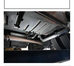
6 With everything in place and sitting with proper clearance begin to tighten the clamps from the front to the back. Tighten each side evenly. We recommend using an impact wrench.
