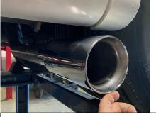
4. Slide the tip onto the Gibson exit pipe. Then install it onto the overaxle pipe, You will do this to help determine the correct height. The tip should be no closer than 1.5"to your RV body panel and stick out no less 1.5" Do not tighten
