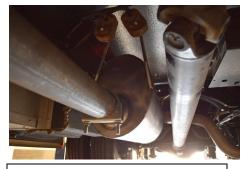
2. Install the muffler onto the factory head pipe and slide into the factory rubber grommets. Do not tighten.
