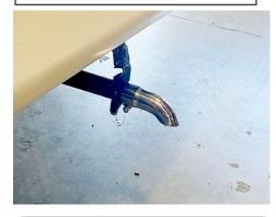
7. To Install the Generator turn down kit simply hold the tip up to your factory exhaust and mark the end of the tip. Add 1.5" to the mark towards the end of the exhaust and cut. Be sure the tip still extends past your body panel 1.5".
