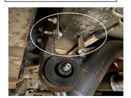
5. You may need to use the provided drop hanger to find the right height. If so, you will un bolt the factory hanger and use the kit to drop it down with the provided hardware.
