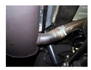
2. To remove the stock exhaust, unbolt band clamp located just behind your factory muffler. Disengage the welded hangers using WD-40 from the OEM rubber grommets. Do not damage or remove the rubber grommets as you will reuse them to mount your new system.
