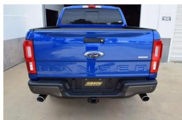
8. INSTALL THE TIPS BY SLIDING THEM OVER EACH EXIT PIPE AND THEN ADJUSTING THEM TO YOUR DESIRED LENGTH AND ROTATION. EXIT PIPES CAN BE ROTATED FOR DESIRE TIP CLEARANCE FROM BUMPER. TIGHTEN ALL CLAMPS STARTING FROM THE FRONT OF THE SYSTEM TO THE BACK.
