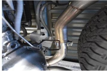
5. NEXT, SLIP A (#I) 2.5" BAND CLAMP OVER THE INLET END OF THE DRIVER SIDE (#C) OVER AXLE PIPE (B) AND INSTALL ONTO END OF DRIVER (#B) OVER AXLE PIPE (A). KEEP CLAMP SLIGHTLY LOOSE FOR ADJUSTMENT
