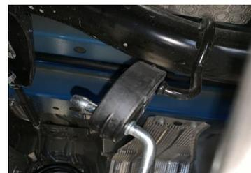
3. INSERT REAR MUFFLER HANGER INTO CORRESPONDING RUBBER GROMMET.
