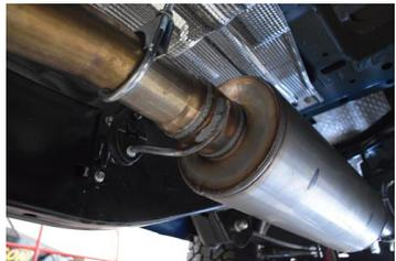
2. SLIDE MUFFLER ONTO THE HEADPIPE 1 1/2" TO 2". SO THAT THE LOCATOR PIN LOCATES INTO THE NTOCH ON THE MUFFLER ASSEMBLY. USE JACK STAND TO SUPPORT THE MUFFLER. ATTACH CLAMP (#H) AT THE INLET OF THE MUFFLER. DO NOT TIGHTEN.
