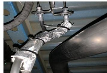
6. NEXT, USING TWO ZIP TIES SUPPLIED IN THE KIT, SECURE THE TWO BRAKE LINE HOSES AWAY FROM OVER AXLE PIPE. LINES MUST BE AT LEAST 1" FROM PIPE. THEN TAKE THE HEAT SLEEVE AND CUT IT LENGTHWISE IN ORDER TO WRAP AROUND BRAKELINES. SECURE WITH REMAINING 3 ZIP TIES.
