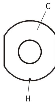
Orient the score mark ( H ) on adjusting head in the center of any of the four sides of the square rod stop. Then lock the parts together by screwing the lock nut up to the adjuster head.
