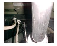
INSTALL BAND CLAMP # I ONTO MUFFLER, INSERT HANGER INTO RUBBER GROMMET, USE BOLT KIT PROVIDED, DO NOT TIGHTEN.
