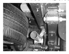
1. TO REMOVE YOUR EXHAUST 2WD- CUT 8" IN FRONT OF YOUR STOCK MUFFLER.
