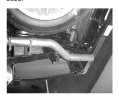
3. INSTALL PASSENGER SIDE OVERAXLE PIPE #C INTO MUFFLER AT LEAST 1  $\frac{1}{2}$ " NO MORE THAN 2". ATTACH WITH HANGER # H AND CLAMP # G.
