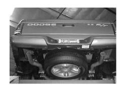
5. INSTALL EXIT PIPE # F TO OVERAXLE PIPES USE CLAMP # G TO SECURE THEM. DO NOT TIGHTEN. ADJUST PIPE TO THE RIGHT ANGLE AND CUT TO LENGTH. IF YOUR VEHICLE HAS A SWAY BAR YOU MAY HAVE TO TRIM THE FACTORY BOLT ON PASSENGER SIDE INSTALL CLAMP # G TO HANGER # I ON BOTH SIDES TO HOLD UP YOUR TAILPIPES.
