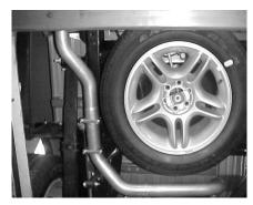
4. INSTALL DRIVERSIDE TAILPIPE PIPE # C INTO MUFFLER AT LEAST 1 ½" NO MORE THAN 2". ATTACH TAILPIPE TO MUFFLER WITH CLAMP # G, AND ATTACH HANGERS # I TO TAILPIPES.NEXT INSTALL OVERAXLE PIPE #E TO FRONT TAILPIPE, USE CLAMP # G TO SECURE PIPES. DO NOT TIGHTEN YET.
