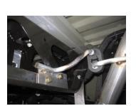
head pipe #A 1.5-2" with louvers facing towards the converter. Use a jack stand to support the muffler. Use clamp #G to secure together. Do not tighten.
