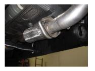
3. Install headpipe #A onto your existing stock 2-bolt flange. Use stock nuts to secure. Do not tighten On short beds cut 12.5" off headpipe
