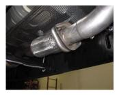
3. Install headpipe #A onto your existing stock 2-bolt flange. Use stock nuts to secure. Do not tighten On short beds cut 12.5" off headpipe
