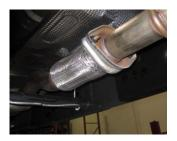
2. To remove your stock exhaust, unbolt the 2-bolt flange located in front of the muffler. For an easier removal of the factory exhaust cut off your tailpipe behind the muffler outlet. Leave all rubber grommets in place. Use WD-40 to aid in the removal of the hangers from the rubber grommets.
