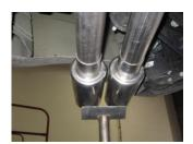
7. Install stainless steel tips. Clamp down. When you have everything in place, firmly tighten all bolts and clamps down securely. Inspect all fasteners after 25-50 miles of operation and re-tighten as necessary.
