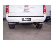
Clamp down. When you have everything in place, firmly tighten all bolts and clamps down securely. Use stainless steel cleaner and a Scotch Brite pad weekly to prevent tip from discoloration.
