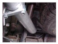
INSTALL DRIVER SIDE TAILPIPE #D INTO MUFFLER AT LEAST 1½" TO 2". THIS PIPE WILL ROUTE OVER THE AXLE AND BETWEEN THE SHOCK AND TIRE. ATTACH CLAMP #G TO SECURE TAILPIPE TO MUFFLER. DO NOT TIGHTEN. INSERT WELDED HANGER INTO RUBBER GROMMET.
