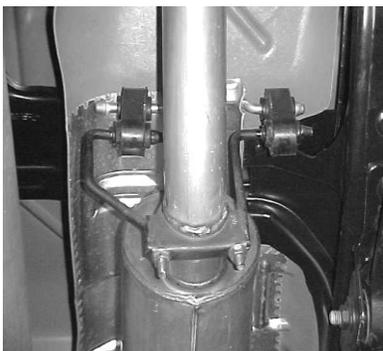
INSTALL HANGER #G ON THE OUTLET OF THE MUFFLER. DO NOT TIGHTEN. INSERT WELDED HANGER INTO RUBBER GROMMET. HANGER WILL BE FACING TOWARDS PASSENGER SIDE FRAME RAIL.
