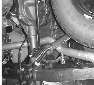
INSERT WELDED HANGER INTO THE RUBBER GROMMET.
