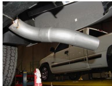
INSTALL YOUR EXITPIPE #D AND USE CLAMP #H TO SECURE THE PIPES TOGETHER. ROTATE THE PIPES UNTIL THEY ARE LEVEL.
