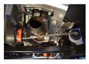
**2.** To install your new Gibson Exhaust, install the supplied headpipe assembly into the factory hangers. Use Bolt Kit.
