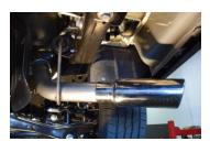
**6.** Lastly, install exit pipe using the last 3" band clamp and adjust according to your desired tip position. Install tip and tighten all bolts and clamps working from the headpipe towards the exit pipe.
