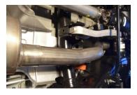
**4.** Install the overaxle pipe into the outlet of the muffler using one of the supplied 3" band clamps.
