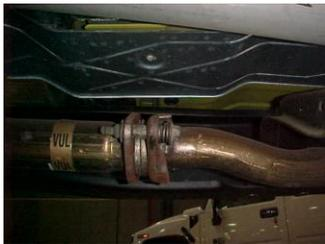
LAY OUT THE EXHAUST AND COMPARE PART NUMBERS. FOR AN EASIER REMOVAL OF THE STOCK EXHAUST CUT THE TAILPIPE BEHIND THE MUFFLER USING A HACKSAW. UNBOLT THE FACTORY FLANGE IN FRONT OF THE MUFFLER WITH OUT REMOVING THE FACTORY DOUGHNUT GASKET. YOU WILL RE-USE STOCK BOLTS. NOW REMOVE YOUR STOCK EXHAUST. LEAVE ALL RUBBER GROMMETS IN PLACE.
