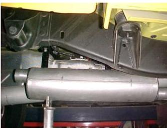
SLIDE MUFFLER #C ONTO THE HEADPIPE 1 1/2" TO 2". THE MUFFLER INLET IS LOOKING INTO THE LOUVERS. USE JACK STAND TO SUPPORT THE MUFFLER. ATTACH CLAMP #G AT THE INLET OF THE MUFFLER. THE MUFFLER OUTLET SHOULD BE POSITIONED AT ABOUT 12 O'CLOCK. DO NOT TIGHTEN
