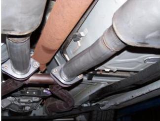
**3.** Install head pipes #A & B onto your existing stock front pipe and attach with factory hardware. Do not tighten.
