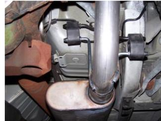
**7.** Install passenger side exit pipe #F onto tailpipe use clamp #I to secure pipes together. Insert welded hanger into rubber grommet. Do not tighten.
