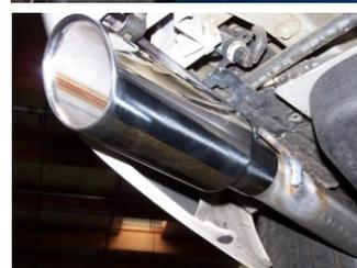
**9.** Install stainless steel tips #H. Clamp down. When you have everything in place, firmly tighten all bolts and clamps down securely. Use stainless steel cleaner and a Scotch Brite pad weekly to prevent tip from discoloration. Inspect all fasteners after 25-50 miles of operation and re-tighten as necessary.
