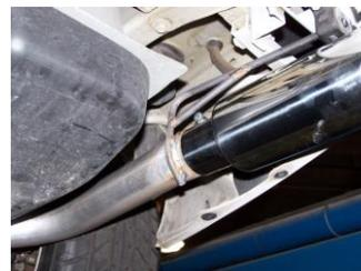
**8.** Install drivers side exit pipe #G. Use clamp #I to secure to the tailpipes together. Insert welded hanger into rubber grommets. Do not tighten.
