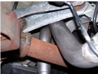
**5.** Install drivers side overaxle tailpipe #E into mufflers 1 1/2" to 2". Insert welded hangers into rubber grommets use clamp #I to secure to muffler. Do not tighten.
