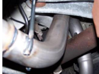
**6.** Install passenger side overaxle tailpipe #D into the muffler 1 1/2"-2". Insert welded hangers into rubber grommets. Use clamp #I to secure tailpipe to muffler. Do not tighten.
