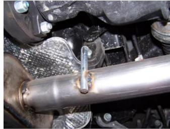
Install passenger side tailpipe assembly #C. Insert all welded hangers into rubber grommets. Secure tailpipe with clamp #D. Do not tighten.
