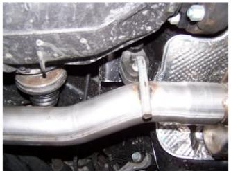
Install driver side tailpipe assembly #B. Insert all welded hangers into rubber grommets. Secure tailpipes with clamp #D. Do not tighten.
