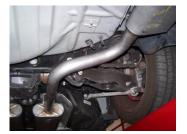
6. Install passenger side tailpipe/muffler assembly #C. Insert all welded hangers into rubber grommets. Secure tailpipe with clamp #D. Do not tighten. Now go back and make sure the first two mufflers in the middle are level.
