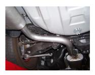
4. Install driver side tailpipe/muffler assembly #B. Insert all welded hangers into rubber grommets. Secure tailpipes with clamp #D. Do not tighten.
