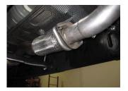
3. Install headpipe #A onto your existing stock 2-bolt flange. Use factory nuts to secure. Leave loose until the whole system is installed. Insert welded hanger into rubber grommet. On short bed cut 12.5" off headpipe.
