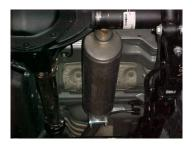
Install muffler #B onto head pipe #A 1-1/2" to 2" with the louvers facing towards the converter. Use a jack stand to support the muffler. Outlet of muffler will be level.
