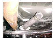
Install head pipe # A on to your existing stock 2-bolt flange use bolt kit #G to secure. Leave loose until the whole system is installed.
