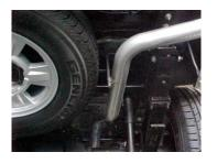
Install drivers side tailpipe # C into muffler 1-1/2" to 2". Rotate until it touches the rear mount, use clamp # H to secure tailpipe to muffler. Do not tighten.
