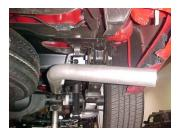
Install exit pipes # E onto tailpipe, use clamps # H to secure pipes together, do not tighten.
