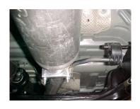
Next install front muffler hanger #E onto muffler. Insert hanger into rubber grommets. Do not tighten.
