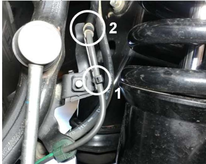
DD. Remove OE ABS line bracket by removing the hex head cap screw with a 10mm socket.
