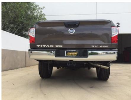
5. Install The Stainless steel tip Item# C onto the exit pipe. Adjust the tip and exit pipe to your desired position.
