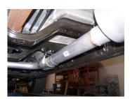
5. Slide resonator #B onto the Y Pipe 11/2"-2". Use clamp #G to secure pipes together. Do not tighten.
