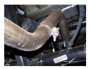
2. To remove your stock tailpipe, remove the clamp shown here. Disengage hanger from rubber grommet. Use WD-40 to aid in this process. Leave all rubber grommets on the factory hangers on the vehicle.
