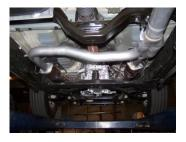
4. Install Y Pipe #A onto the stock flanges using the stock gaskets and hardware. Do not tighten. Insert welded hanger into rubber grommet.
