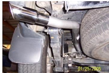
INSTALL THE STAINLESS STEEL TIP. TO CLEAN TIP USE ANY STAINLESS OR ALUMINUM CLEANER AND A SCOTCH BRITE PAD. NOW GO BACK AND TIGHTEN ALL CLAMPS, NUTS AND BOLTS STARTING FROM THE FRONT AND WORKING YOUR WAY BACK.
