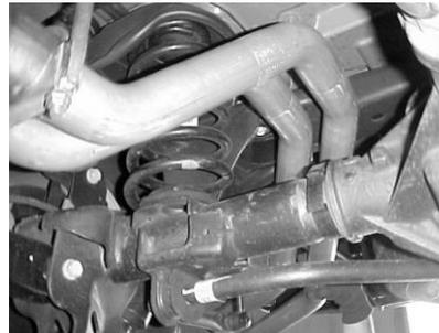
INSTALL DRIVERSIDE TAILPIPE # C INTO OUTLET OF MUFFLER, 1-1/2" TO 2". REAR MUFFLER HANGER #E WILL BE USED TO SECURE PIPE TO MUFFLER. DO NOT TIGHTEN.
