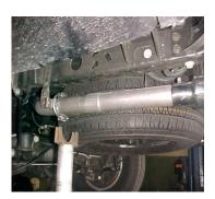
USE CLAMP # I TO SECURE TO THE MUFFLER, INSERT WELDED HANGER INTO THE RUBBER GROMMET. DO NOT TIGHTEN. NEXT, INSTALL THE EXIT PIPES # E AND #F. USE CLAMPS # H TO SECURE TO THE TAILPIPES. DO NOT TIGHTEN. USE ZIP TIES TO SECURE BRAKE AND FUEL LINES AWAY FROM EXHAUST.
