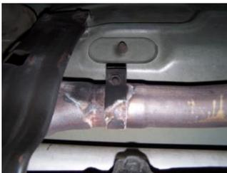
4. Then unbolt head pipe at clamp and remove.
