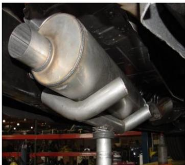
INSTALL MUFFLER # B ONTO TAILPIPE 1-1/2" TO 2" WITH INLET TOWARDS THE MOTOR. USE CLAMP # F TO SECURE THE TAILPIPE AND THE MUFFLER, DO NOT TIGHTEN. INSERT WELDED HANGER INTO RUBBER GROMMET ON THE TAILPIPE. MUFFLER INLET SHOULD BE AT 9 O'CLOCK POSITION.
