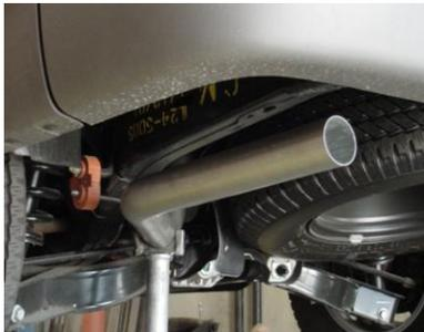
INSTALL EXIT PIPE # D AND INSERT WELDED HANGER INTO RUBBER GROMMET.
