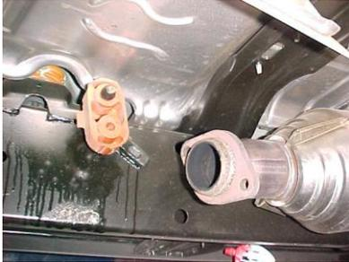
TO REMOVE STOCK EXHAUST UNBOLT IT FROM THE SLIP-FIT JOINT LOCATED IN THE REAR ABOVE THE AXLE AND SLIDE THE TAILPIPE OUT. NEXT UNBOLT THE 2-BOLT FLANGE LOCATED JUST BEHIND THE CATALYTIC CONVERTER. **DO NOT THROW AWAY STOCK NUTS AND BOLTS YOU WILL NEED TO RE-USE THEM.** LEAVE ALL RUBBER GEOMMETS ON THE HANGERS. USE WD-40 TO AID IN THE REMOVAL OF EXHAUST AND HANGERS.
