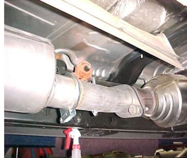
INSTALL HEADPIPE #A. SLIDE HEADPIPE INTO MUFFLER 1-1/2" TO 2" USE CLAMP # F TO SECURE HEADPIPE TO MUFFLER. DO NOT TIGHTEN. NEXT USE YOUR STOCK NUTS AND BOLTS TO SECURE HEADPIPE TO STOCK FLANGE.
