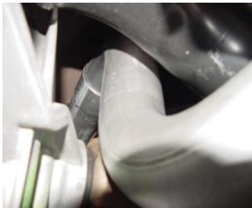
INSTALL THE STAINLESS STEEL TIP. TO CLEAN TIP USE ANY ALUMINUM OR STAINLESS CLEANER AND A SCOTCH BRITE PAD. GO BACK AND TIGHTEN ALL NUTS, BOLTS AND CLAMPS STARTING IN THE FRONT AND WORKING BACK.
