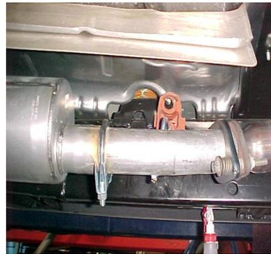
INSTALL TAILPIPE # C. SLIDE IT INTO THE EXITPIPE # D, USE CLAMP #F TO SECURE THE TAILPIPE TOGETHER. DO NOT TIGHTEN.
