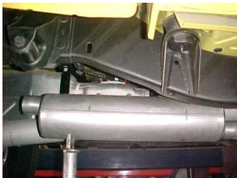
SLIDE MUFFLER #C ONTO THE HEADPIPE #A 1 1/2" TO 2". THE MUFFLER INLET IS LOOKING INTO THE LOUVERS. USE JACK STAND TO SUPPORT THE MUFFLER. ATTACH CLAMP #G AT THE INLET OF THE MUFFLER. THE MUFFLER OUTLET SHOULD BE POSITIONED AT ABOUT 12 O'CLOCK. DO NOT TIGHTEN
