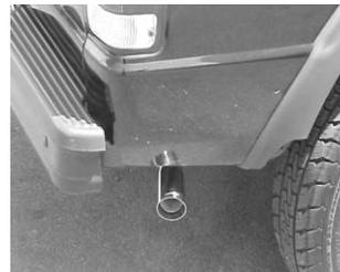
INSTALL THE STAINLESS STEEL TIP. USE ANY ALUMINUM OR STAINLESS STEEL CLEANER TO POLISH THE TIP. NOW TIGHTEN ALL CLAMPS, HANGERS, AND BOLTS.
