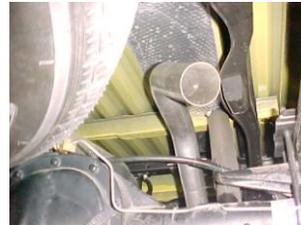
INSERT THE OVERAXLE TAILPIPE #D INTO THE OUTLET OF THE MUFFLER 1 1/2" TO 2" INTO THE MUFFLER AND ATTACH USING CLAMP #H. DO NOT TIGHTEN
