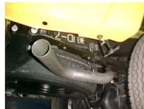
SLIDE TURN OUT PIPE #E ONTO THE OVERAXLE PIPE. INSERT WELDED HANGER INTO FACTORY RUBBER GROMMET. USE CLAMP #G TO ATTACH PIPES TOGETHER. DO NOT TIGHTEN.
