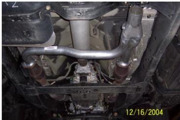
INSTALL Y-PIPE # A & I ONTO STOCK FLANGES USE YOUR STOCK HARDWARE TO SECURE. INSERT WELDED HANGER INTO RUBBER GROMMET, DO NOT TIGHTEN.
