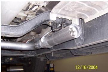
NEXT, INSTALL RESONATOR # B 1 1/2"-2" ONTO Y-PIPE USE CLAMP # G TO SECURE PIPES TOGETHER, DO NOT TIGHTEN.
