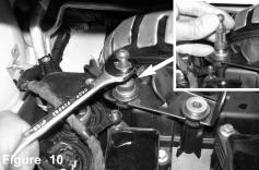
Now loosen the engine cover fitting using 12mm wrench. Remove and save fitting and grommet with spacer for later install
