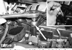
Loosen the 8mm screw holding in the plastic turbo elbow. Remove the screw.
