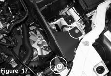
Once fitted properly, secure and tighten both screws using 10mm socket and wrench.
