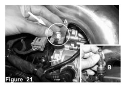
A)Install the primary intake tube and secure to the turbo nut and fender washer. B)Re-install the fitting from step10, this will allow for the engine cover install.
