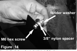
Locate the hole on heat shield, install the hex screw through heat shield, now attach the nylon spacer than the fender washer.
