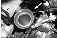
Install the step hose to the turbo with clamps provided. Tighten the clamp on the turbo only. Place clamp on the 3" 11. Secure and make sure the seal seats and the clip side in a spot allowing for easy access when you tighten
