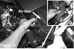
A)Lift up and carefully remove the stock air box. B)Now remove the rubber snorkel sleave.
