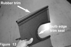
Install the bulb edge trim to the cut out on heat shield. Install the rubber trim to the top of the heat shield.
