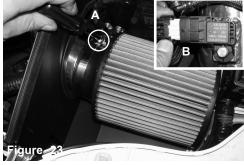
A)Install the air filter. Position the intake for the best fit, secure the vibramount using 10mm socket or wrench. B)Connect the temp sensor. Re-install the engine cover. Connect the battery terminals.
