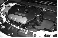
Stock air box assembly shown in this picture. Disconnect pattery before the install. Remove the engine cover.
