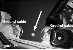
Install the heat shield into the vehicle. Locate the thredded insert on the frame . Make sure the spacer is installed. secure the heat shield.
