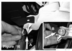
Secure the heatshield tab to the factory position air box bracket. Install the hex screw with fender washer bottom up. Secure the top of the tab using provided M6 nut and fender washer.
