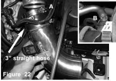
A)Attach the 3" straight hose with clamps to the primary and bracket to the vibramount. Secure using provided m6 intake tube. Now install the secondary tube and connect to tighten all clamps using 8mm nut driver. Tighten and the primary tube. Do not tighten.B)Connect the crankcase line to the engine fitting.
