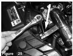
Tighten using 10mm socket and ratchet.
