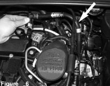
Disconnect the crank case line from engine and remove from vehicle.
