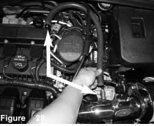
Install the 15mm vacuum line to the engine and to the fitting on the intake tube.
