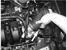
Pull back intake tube from throttle body.
