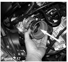
Install the step hose to the throttle body with clamps provided. Tighten the throttle body clamp only.
