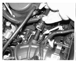
Disconnect the crank case line from the stock intake.
