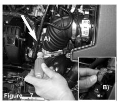
A) With 8mm nut driver, loosen the clamp on throttle body. B) Disconnect the MAF sensor harness.
