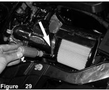
Re-position the filter shield to desired position, make sure that its not touching anything.
