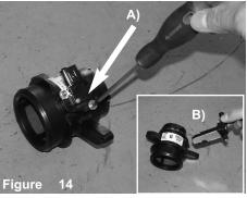
A) WithT20 torx screwdriver, loosen the 2 screws holding in the MAF sensor. B) Carefully remove the MAF sensor from the housing.
