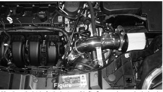
Align the entire intake for the best possible fit. Once you have rechecked and cleared the intake from all moving parts, continue to tighten all nuts, bolts and clamps.
