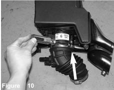
Loosen the clamp on the air box using 8mm nut driver and remove the stock intake tube.
