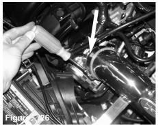
Tighten the clamps using 8mm nut driver..
