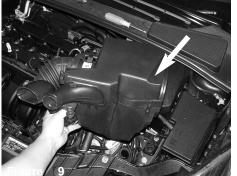
Pull back the ram air scoop from radiator support. Carefully lift and pull out air box.
