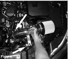
Install the intake assembly into the the vehicle and position to throttle body and bracket to vibra mount.
