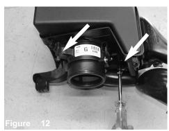
Loosen the 2 screws holding in the MAF sensor housing using 8mm nut driver.
