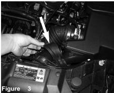
Pull back the rubber clamp holding in the air box to the front of the radiator support.
