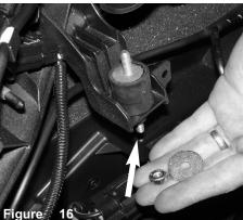
Position for the best fit, and secure using provided M6 washer and nut. Tighten using 10mm socket or wrench.
