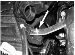
Position the bracket on the vibra mount and secure using provided M6 washer and nut.
