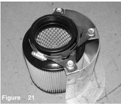
Slide the filter into the middle and position clamp over the composite clamps. Make sure the clamps sit over the bead on the filter. Tighten bolts using13mm socket.
