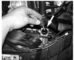
Attach the longer side of the provided vibra mount to the factory hole tab located in front of the raditator support.
