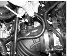
Disconnect the vacuum line from stock intak.
