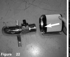
Install the filter to the intake tube and tighten.
