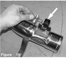
Secure and tighten the MAF sensor using provided M4 button head screws using 2.5mm allen key.
