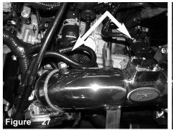
Connec the Vacuum line to the fitting on the intake
