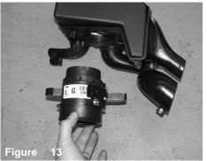
Carefully remove MAF sensor housing from air box.
