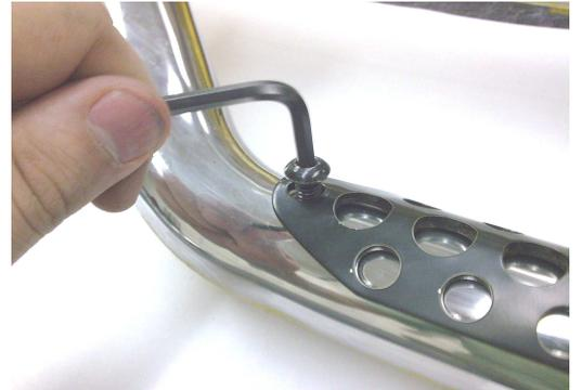
2. Apply a fine cleaning solution to a clean cloth. Gently wipe away all dust, mud, and salt from the inside of the step pad nutsert. Avoid dropping any liquid directly into the nutsert. Protect the finish by applying a non-abrasive wax (e.g. pure carnauba).
