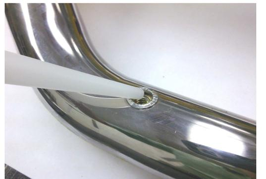
5. Replace the aluminum step pads and tighten the bolts back into place using the 5/8" hex tool.
